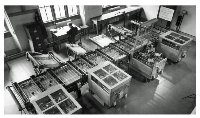
The differential analyzer: a brain the size of a room that could whir away at a problem for days and nights on end. "It was a fearsome thing of shafts, gears, strings, and wheels rolling on disks—but it worked."
